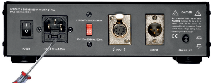
Figure 4: Opening the fuse compartment
