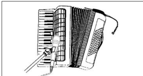
Fig. 7: Miking up an accordion with a C 516 ML and a stand-mounted microphone.
