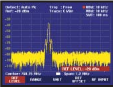
Microphone A carrier frequency Spectrum analyzer trace
