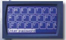
As with the SW9010, up to 100 control 'pages' of virtually any Soundweb London DSP parameter can be constructed, with the ability to create 'folders' for nested menus. Access to specific pages can be restricted with the used of password protection, so that only engineers or key employees can adjust critical system parameters.
