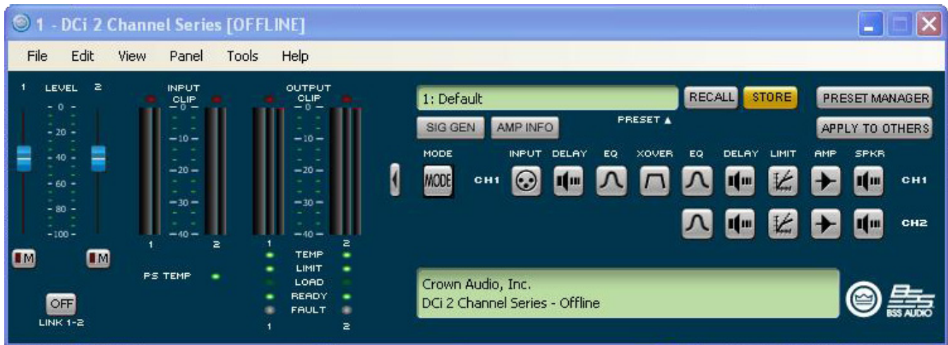
Figure 10 With the "Y 1+2" box checked, both output Ch.1 and Ch.2 are fed by input Ch.1 and input processing is organized accordingly.
