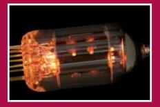
The dual-triode circuitry of the ECC 83 tube of the AKG P 820 Tube boosts the even-order harmonics for a rich and "warm" sound.
