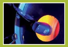
The engineers at the AKG acoustic research laboratory tested the P 2 with many different kick drums. To get the best possible sound, they recommend a 3 dB boost at 70 Hz and a 3 dB cut at 700 Hz on the EQ (e.g., on the mixer).
