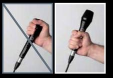
Microphones with cardioid or hypercardioid polar pattern are the most frequently used mics on stage. It is very important to hold the microphone correctly. Take care not to cover the sound inlet basket with your hand, as this will have an unfavourable effect on the polar pattern, while also increasing feedback risk quite considerably.
