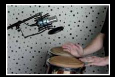
As percussion instruments are beaten by hand, the rapid movements may give rise to irritating wind noise. This can be prevented by installing a windscreen and/ or pop filter between the instrument and the microphone.
