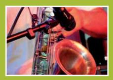
Always place the microphone as close to the sound source as possible! This minimizes the amount of unwanted sound (e.g. from other instruments) picked up by the microphone.
