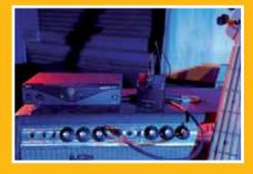
Radio waves are similar to light. Therefore, always place the receiver clear of any potential visual obstructions and wear the bodypack on the guitar strap or on the outside of your clothes so it can always "see" the receiver.
