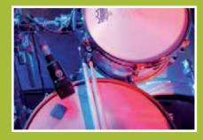
Place the microphone so that it points away from the hi-hat in order to minimize leakage from the hi-hat into the snare drum channel.
