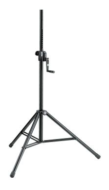
A high quality steel speaker stand with zinc die-cast clamps for professional use. Infinitely variable height adjustment with a hand crank and push button system which prevents an uncontrolled reverse motion. There is an additional locking screw for extra safety. Extension tube diameter 35 mm, suitable for speakers and lighting crossbars with an integrated M10 thread connector.
