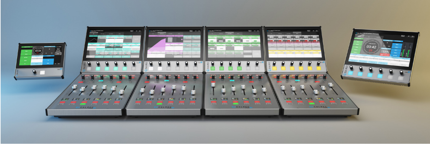
Type R's physical control system consists of just three slimline panels: a fader panel, a large soft panel and a small soft panel. Each is compatible with COTS hardware and powered over ethernet to keep cabling to a minimum.
